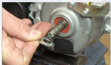
Loosen potentiometer fixing screws, and retrieve the relevant seal
