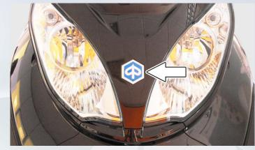
Undo the screw under the badge and remove the centre headlight cover
