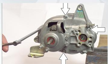
Vice casing and, using a rubber mallet, separate the two half-shells
