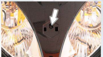
Undo the screws "A" fastening the front grille
