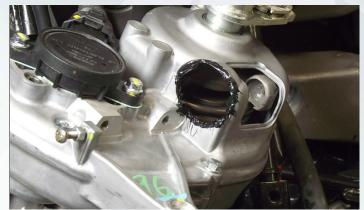
Apply the recommended sealant onto pump body
