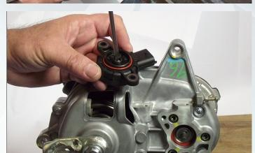
Check for O-ring correct positioning
