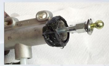
Position pump into its seat, by temporarily tightening fixing screws
