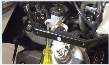
Disconnect gear motor electrical connector
