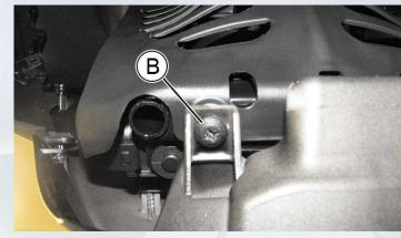
On both sides of the vehicle, undo the screws
