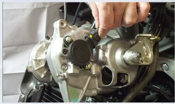
Temporarily connect gear motor
