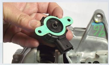
Position potentiometer inside its seat, taking care not to damage drive gear
