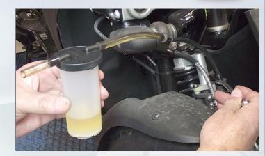
Enable suspension block, and open bleed screw
