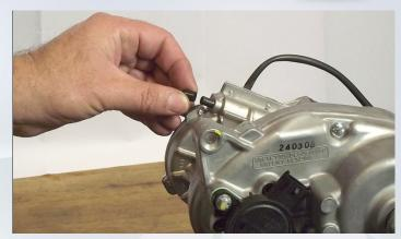
Turn gear motor counter clockwise, until wrench can be inserted in the shown screw
