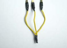
For Quasar injection, Master and 850 twin cylinder stators connection must be done with the three cables connected with terminals. The connection is easily done using the cable assembly of an old regulator.
