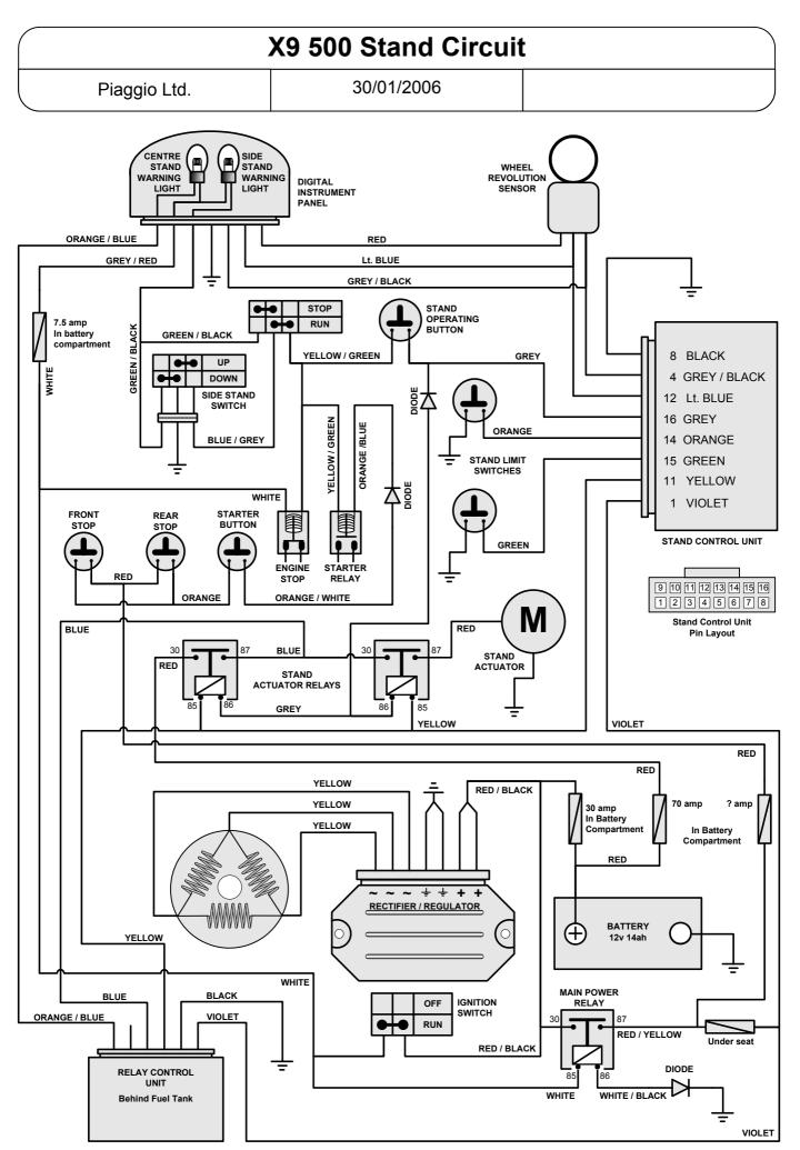
There are two DIODES situated under the front cover above the headlight unit. They are together in black heat shrink tubing There is a single DIODE in the grey wire.
