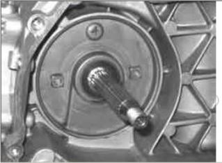
Install the base of the specific tool on the oil guard, using the supplied screws
