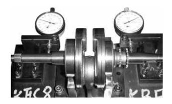
Measure the crankshaft bearing play. **Service Limits:**
