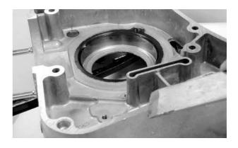
Install a new oil seal into the left crankcase.
