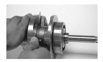
Measure the connecting rod small end I.D. **Service Limit**: 17.06mm replace if over
