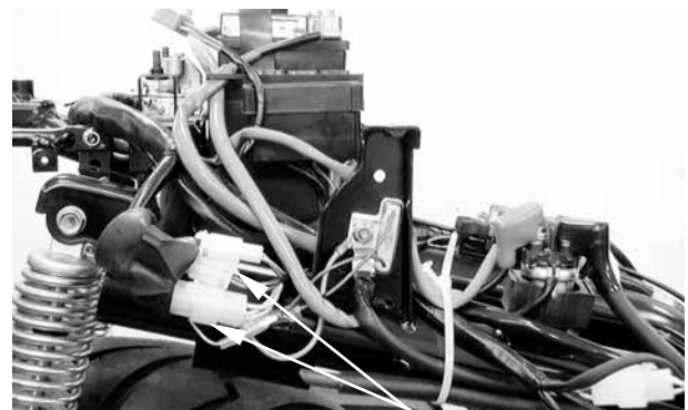
A.C. Generator Wire Connectors Nut Starter Motor Wire
