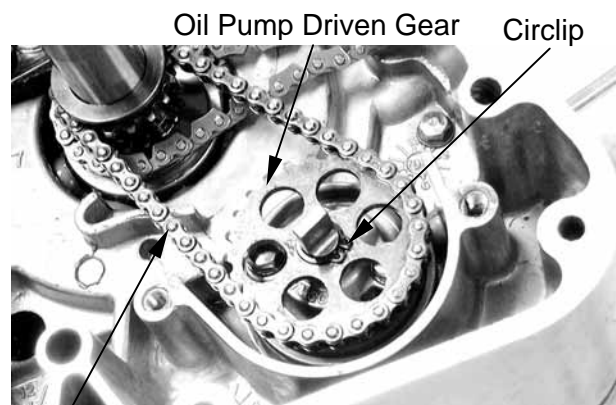
Oil Pump Drive chain
