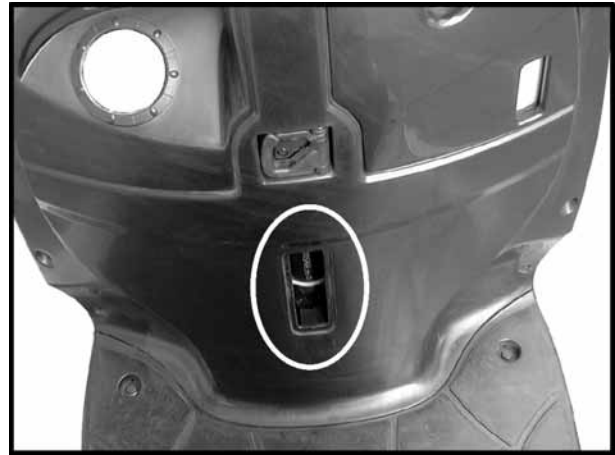
Location of Frame Serial Number
