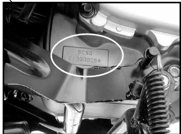
Location of Engine Serial Number
