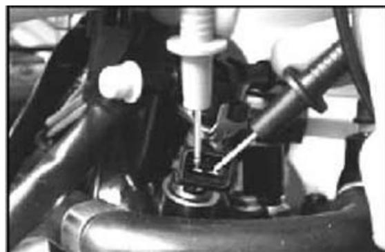
**19** - Check the earth insulation of the injector negative line. Disconnected control unit and injector connectors.
