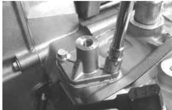
**Locking torques (N\*m)****Tightener fastening screws: 11 ÷ 13**
