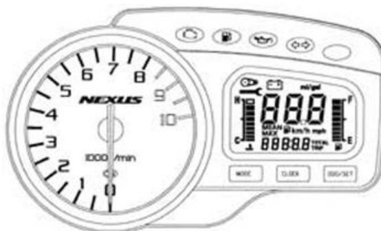
The digital section of the instrument panel is completed by a liquid crystal display and 3 control buttons (MODE - CLOCK - ODO/SET).
