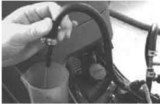
**17** - Introduce the return pipe into a graduated container.
