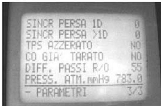
4 - The ambient pressure signal is correct.
