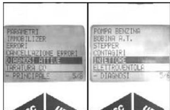
**2** - Enable the function with continuous power supply on and engine off. The control unit controls the fuel pump continuously and at the same time starts the injector opening. The injector openings are repeated for a few seconds.
