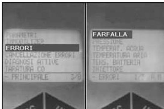
**2** - Select the diagnostic tester menu on the "**PARAMETERS**" function.
