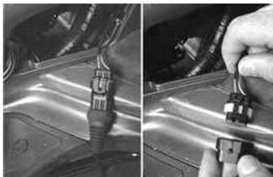
Power the diagnostic tester by connecting the terminals to the battery poles, or the specific connector to the socket inside the gloves compartment.
