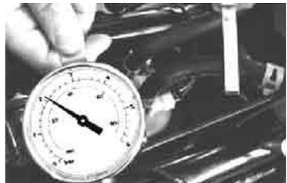
**16** - Disconnect the pump connector, start the engine, wait until it stops and connect the connector again.
