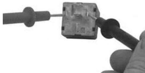
**18** - Check the efficiency of the 10 A fuse no. 2
