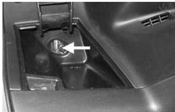
Remove the light, disconnecting the electric connector from the light and the complete lamp holder of the position light.
