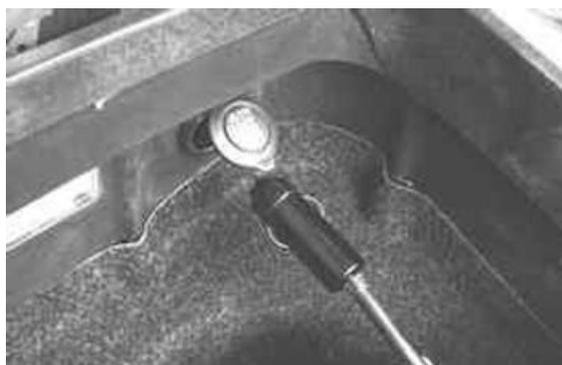
Set the switch to "ON" and select the diagnostic tester menu to the immobiliser function.
