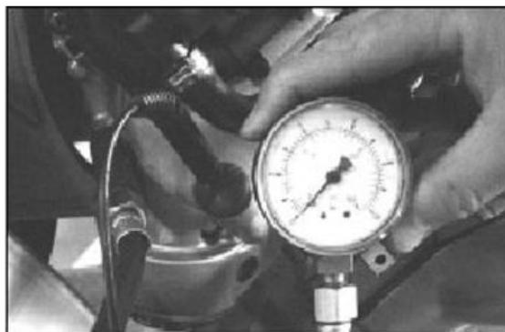
5 - Measure the pressure with cold and idling engine.
