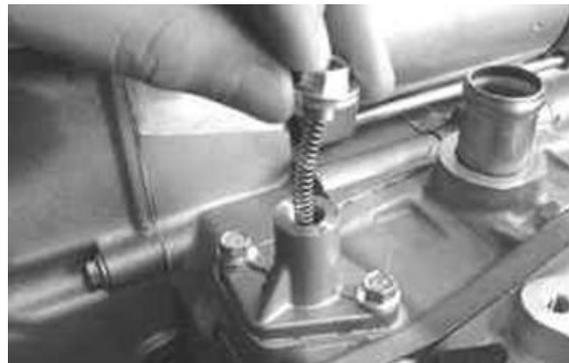
**Locking torques (N\*m)****Tightener screw: 5 - 6**
