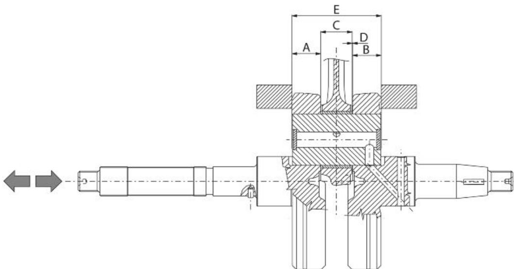
**AXIAL CLEARANCE BETWEEN CRANKSHAFT AND CONNECTING ROD**
