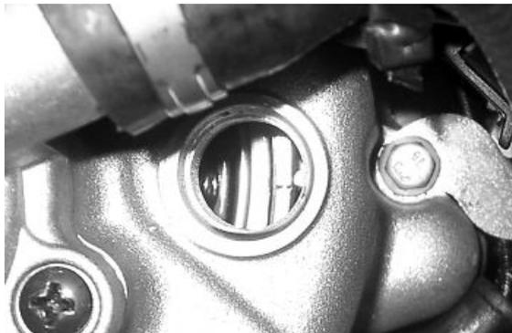
For the use of this reference mark, remove the spark plug and turn the engine in the direction that is the reverse of the normal direction using a calliper spanner applied to the camshaft command pulley casing.
