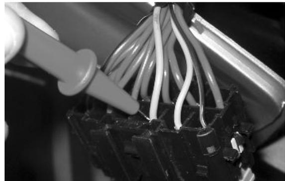
Check there is voltage between pins 22 and 26 of the interface wiring for around two seconds when switching to «ON».
