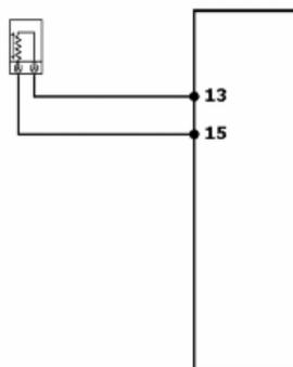
With wiring disconnected from the control unit and connected to the system, check that the sensor resistance between pins 13 - 15 is between 100 and 150 Ohm at an engine temperature of approximately 20°
