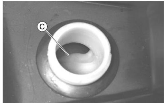
Reference «C» shows the adequate coolant level.
