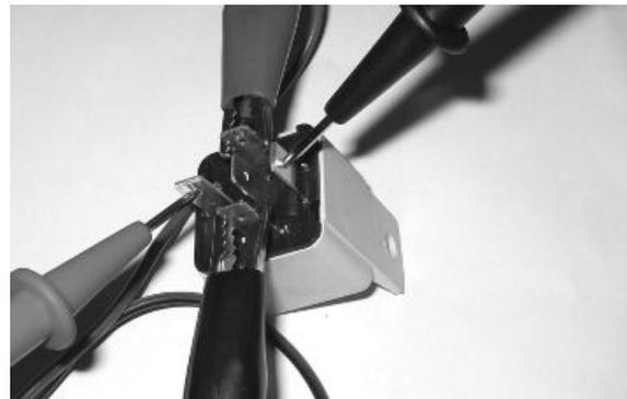
Check the power supply line of the injection load remote control energising coil: After switching to "ON", make sure there is battery voltage, for two seconds, between the black/white cable and black-violet cable of the remote control base. If there is not, check the continuity of the black/white cable between fuse block and the remote control base and of the black/violet cable between pin 20 of the control unit and the remote control base.
