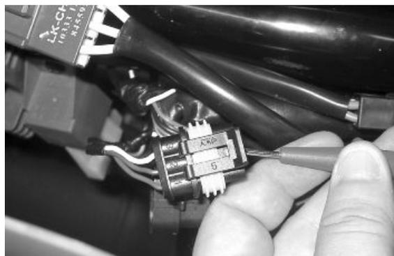
With the revolution sensor connector disconnected and interface wiring disconnected from the control unit, check that the red and white cables (pins 13 - 15) are isolated from each other and insulated from the ground connection.
