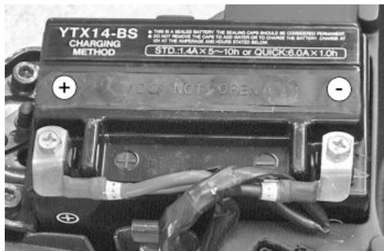
Make sure that the terminals are connected correctly. When a new battery is installed, the correct time and date must be reset on the digital instrument panel («Clock» and «MODE button» section).
