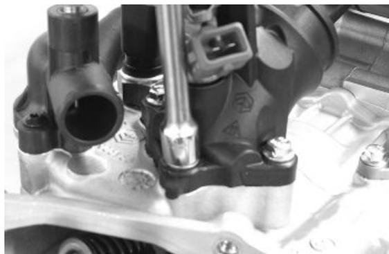
Loosen the three screws and remove the air intake manifold.
