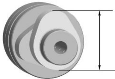
Check the axial clearance of the camshaft
