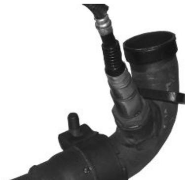
**CAUTION: SHOULD IT BE NECESSARY TO REMOVE ONLY THE MUFFLER TIP, ALWAYS REPLACE THE GRAPHITE GASKET BETWEEN STUB AND TIP.**
