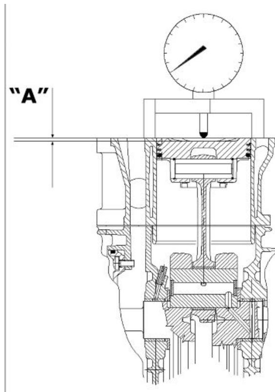
Measurement "A" to be taken is a value of piston re-entry, it indicates by how much the plane formed by the piston crown falls below the plane formed by the top of the cylinder. The further the piston falls
