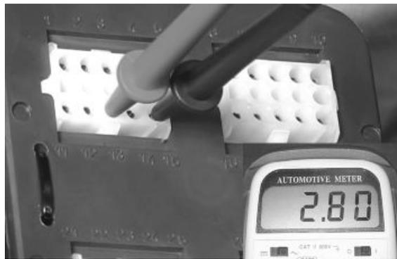
With the interface cabling disconnected from the control unit, check for continuity between pin 13 and the red cable of the rev sensor connector and between pin 15 and the white cable of the rev sensor connector.
