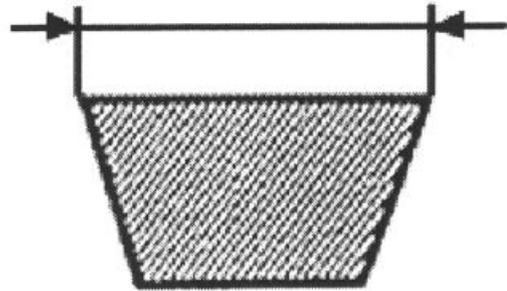
During the wear checks in the scheduled servicing programme, you are advised to check the rim bottom of the tothing does not show signs of incisions or cracking (see figure): The rim bottom of the tooth must not have incisions or cracking; if it does, replace the belt.
