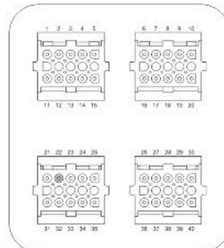
Check the resistance of the primary coil between pin 22 of the interface wiring and the green black cable of the injection load remote control base with the control unit disconnected and the remote control disconnected.
