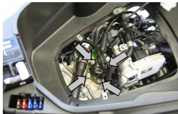
Install the appropriate tool for checking fuel pressure and position the manifold over a container graduated by at least 100 cm<sup>3</sup>. Connect the injector with the cable making up part of the supply for the injection tester. Connect the clamps of the cable to an auxiliary battery. Activate the fuel pump with the active diagnosis. Check that, within fifteen seconds, approximately 40 cm<sup>3</sup> of fuel is dispensed with an adjustment pressure of approximately 2.5 BAR.
