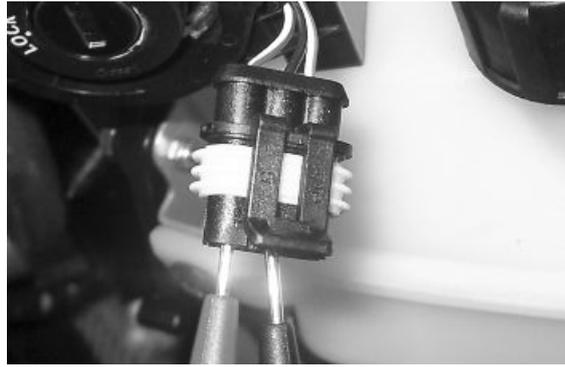
With MIU connector disconnected, check the continuity between the Orange-White cable and pin 7 of the interface wiring .
