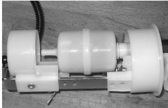
Remove the filter from the pump support
