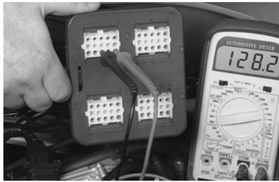
Disconnect the fuel pipe connector. Start up the engine and wait for it to stop. With the wiring connected to the control unit and system try to start up the engine and check that the voltage between pins 13 and 15 is around 2.8 V
