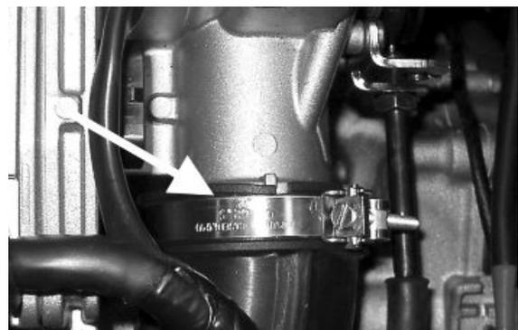
Remove the throttle control retainers as indicated in the photograph.
