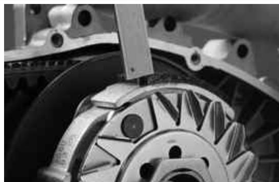
DO NOT OPEN THE MASSES USING TOOLS TO PREVENT A VARIATION IN THE RETURN SPRING LOAD.
