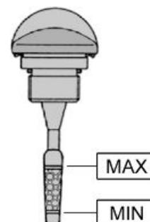
few minutes and switch it off: after five minutes check the level and if necessary top up without exceeding the **MAX** level. The cartridge filter must be replaced every time the oil is changed. Use new oil of the recommended type for topping up and changing purposes.
