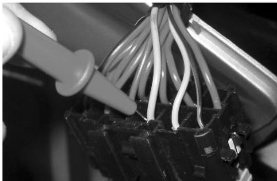
After switching to «ON» and for about 2 seconds, check that there is battery voltage between the Black-Green cable of the pump connector and the ground lead with the pump connector disconnected. Otherwise, check the continuity of the Black-Green cable between the pump connector and the remote control base.
