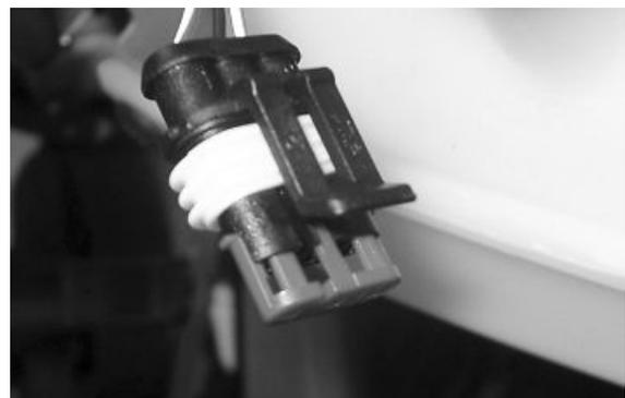
With the ignition key switch set to ON, check if there is battery voltage between the White-Black and Black cables.
