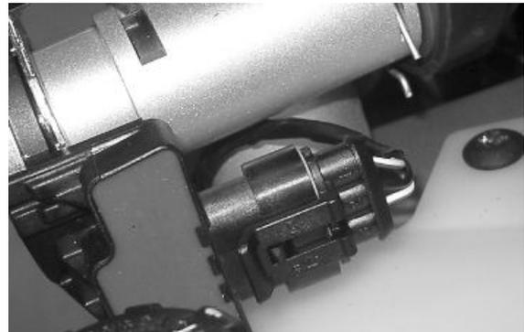
Remove the protective base from the connector.
