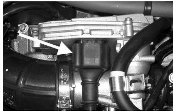
Remove the clip fixing the throttle body to the air cleaner bellows.
