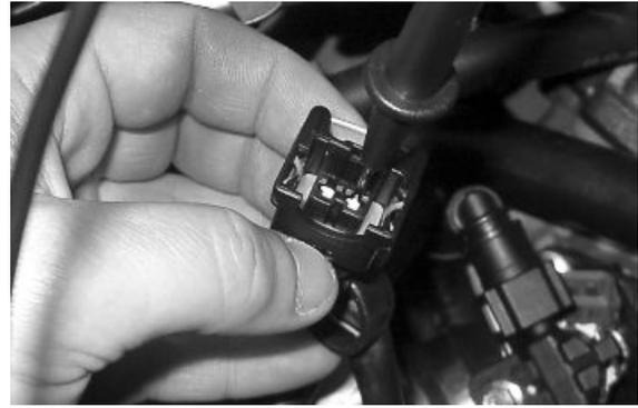
Switch to «ON» and check if there is voltage, with injector disconnected and control unit connected, between the Black-Green cable of the injector connector and the ground lead
