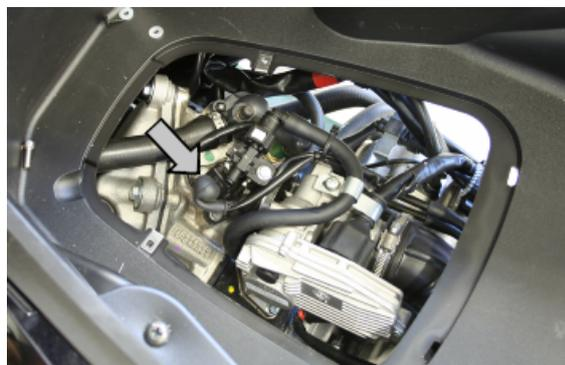
Remove the three screws fixing the manifold to the cylinder head and the clip fixing the throttle body to the manifold.
