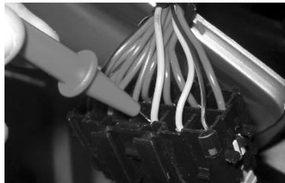
With the control unit and the injector disconnected, check the continuity of the Red-Yellow cable between pin 14 of the interface wiring and the injector connector
