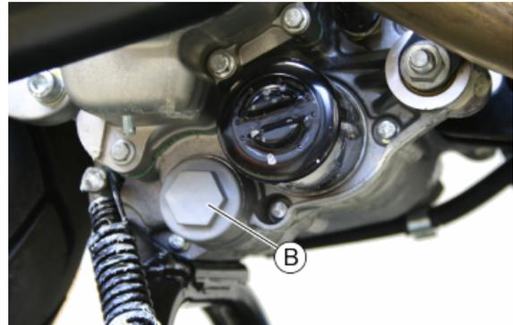
To facilitate oil drainage, loosen the cap/dipstick «A».
