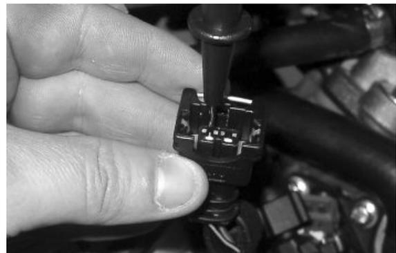
With injector disconnected and the injector load remote control disconnected, check the continuity of the Black-Green cable between the injector connector and remote control base.
