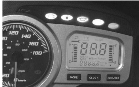
The digital section of the instrument panel is completed by a liquid crystal display and 3 control buttons (MODE - CLOCK - ODO/SET).
