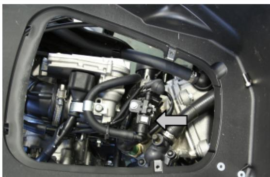
Check during regular operation by placing the appropriate tool between the pump and the injector. With the battery voltage > 12 V check that the fuel pressure is 2.5 BAR and that the input current is 1.4 to 1.8 A
