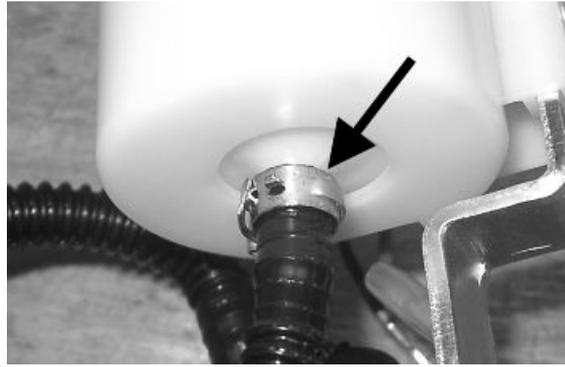
Separate the lower part of the pump support as shown in the photograph.
