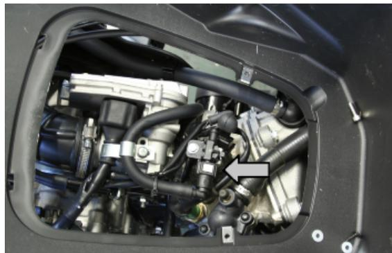
Remove the injector connector.
