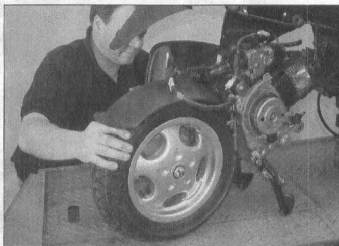
5.8c . . . and manoeuvre the engine out
