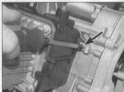
8.5c Rear cowling half is secured to crankcase. Note the clip (arrowed)
