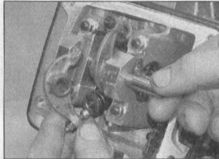
10.4b ... and remove the rocker arms
