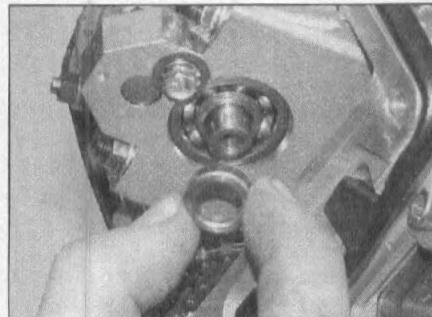
9.5c . . . and remove the spacer
