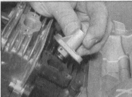
9.12 Install the tensioner . . .
