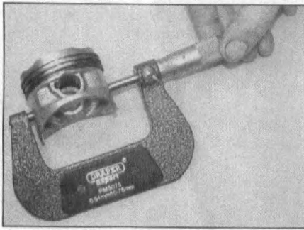
16.8 Measuring the piston diameter
