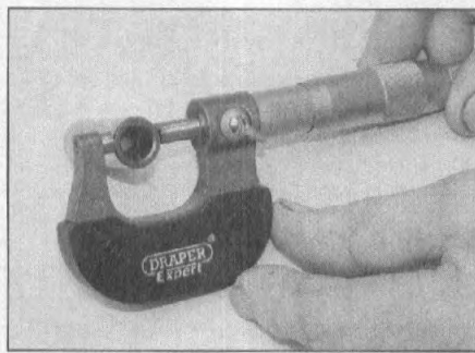
16.9a Measure the piston pin diameter at each end . . .
