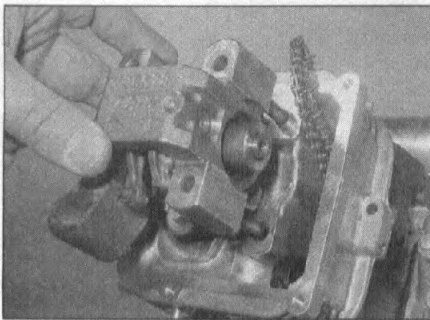
11.5c ... and remove the holder
