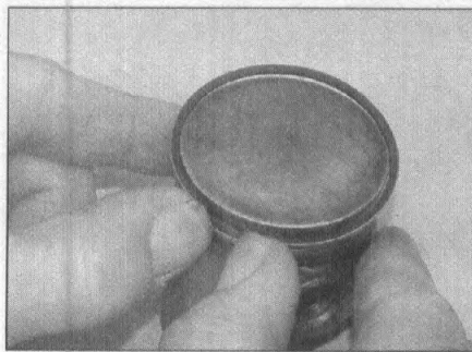
9.5a Remove the piston rings carefully using your thumbs ...
