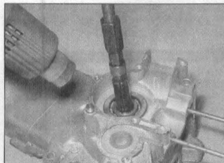
15.6 Using a hot-air gun and internal bearing puller to remove the bearing
