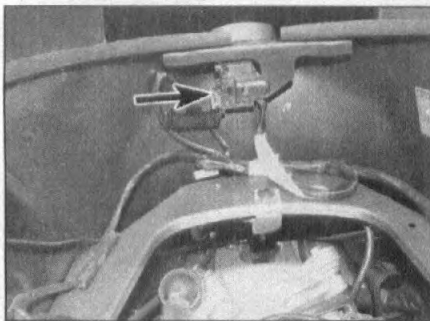
5.1g Location of main fuse (arrowed) ...
