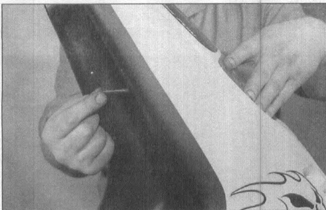
8.2a On the Typhoon, remove the screws ...
