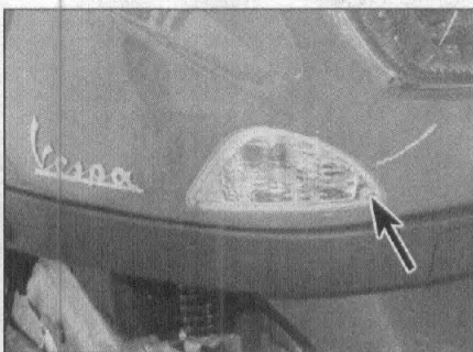
12.10b On LX models remove the screw (arrowed) . . .
