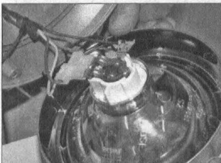
7.1c . . . and disconnect the wiring to free the headlight from the shell
