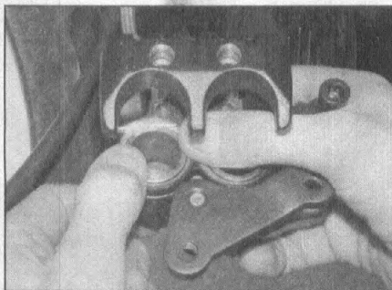
2.22 Push the pistons back into the caliper
