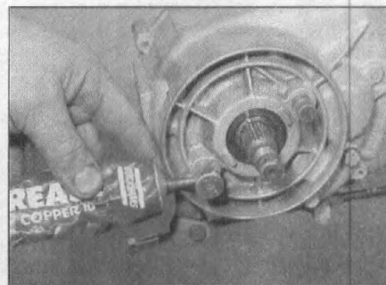
9.11a Apply some copper grease to the cam
