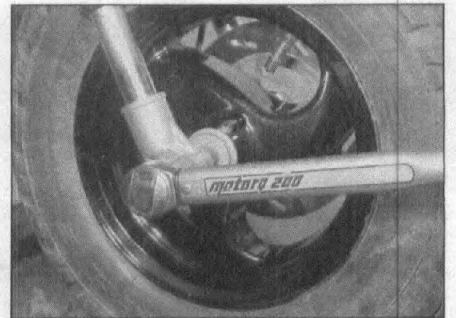
13.19b . . . and tighten it to the specified torque
