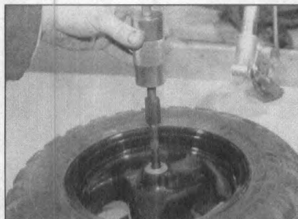
15.18a Using a puller to remove the seals and bearings
