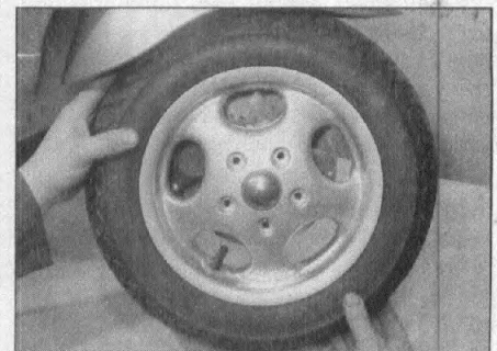
13.2b ... and remove the wheel
