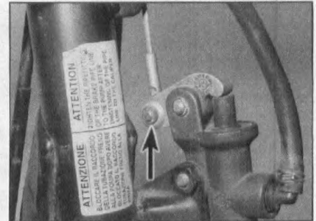
5.16 Remove the E-clip and draw out the pin
