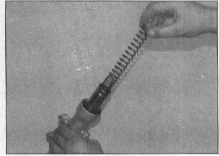
5.61 Compress the fork leg and remove the spring
