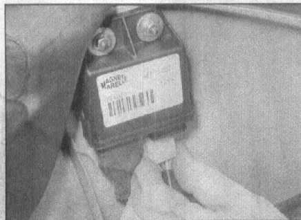
4.2b Disconnecting the pulse generator coil wiring on ET4
