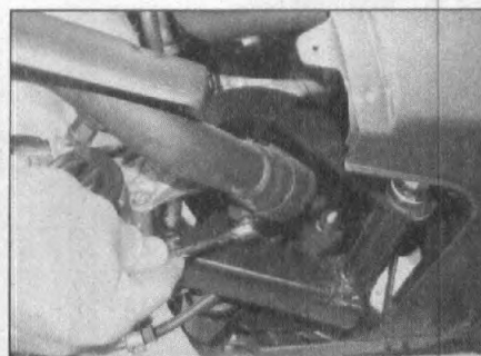
11.3a Loosen the silencer clamp
