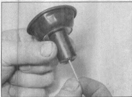
8.4b Push the needle up from the bottom
