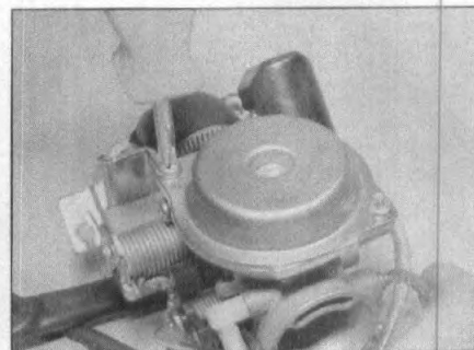
8.3a Remove the screws and the cover ...
