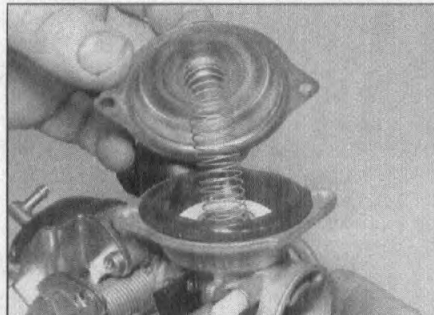
8.30 Locate the cover onto the spring and fit it onto the carburettor
