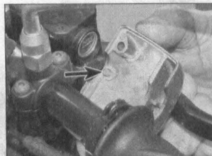
10.12c ... noting how the pin (arrowed) locates in the handlebar
