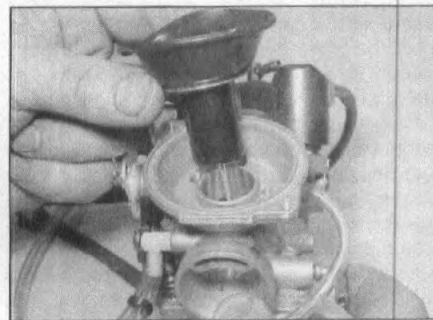
8.3c ... and the diaphragm/piston assembly
