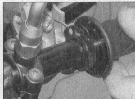
10.12b ... then detach the cable nipple from the twistgrip ...
