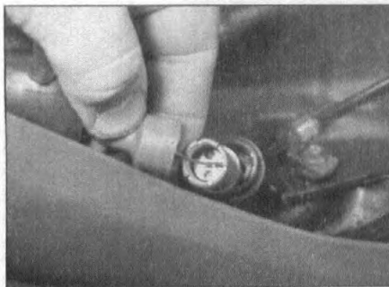
10.8d ... and draw out the slider
