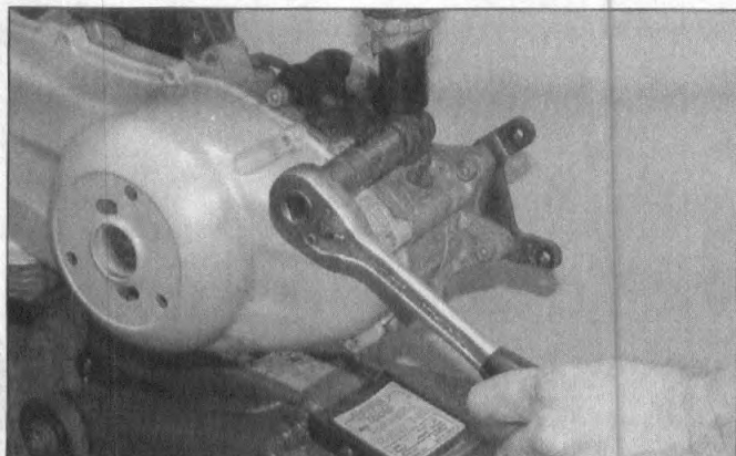
5.8a Undo the lower shock mounting bolt . . .
