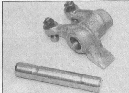
10.5b Keep each rocker arm and its shaft together
