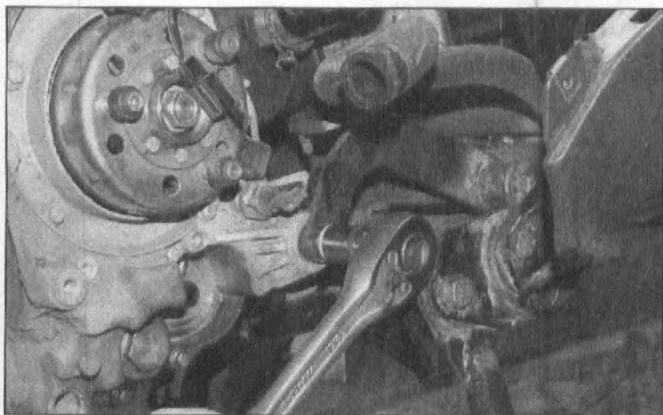
5.7a Undo the nut on the front mounting bolt . . .
