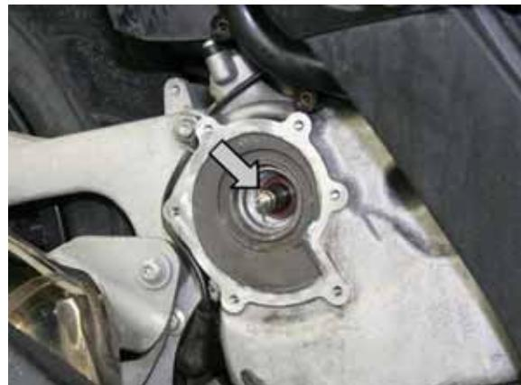
Fit the rod and screw it on the rotor shaft.
