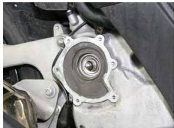
Position the extractor including the pin on the ceramic seal.
