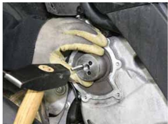
Attach the extractor to the static part of the seal, using the screws including in the tool kit.
