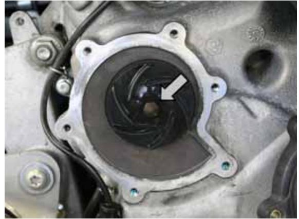
Place two flat blade screwdrivers as shown in the figure to pry on the highlighted edge of the crankcase. Disassemble the integral seal, forced-fitted on the rotor.
