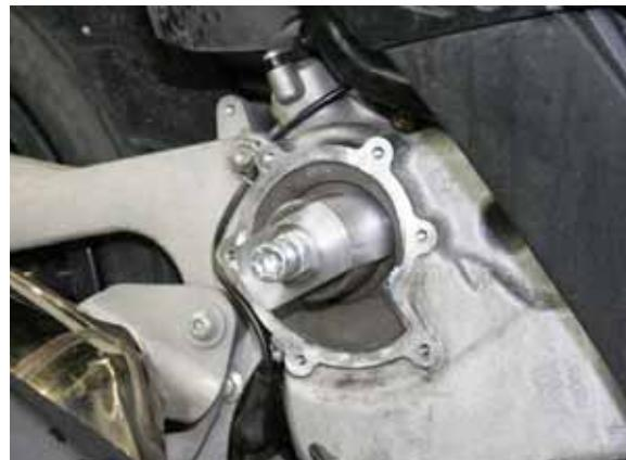
Keep the screw in place and operate on the nut until the fixed section of the seal is pulled out.
