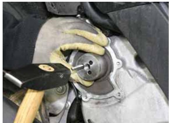
Fix the puller to the fixed section of the seal using the screws supplied with the tool.
