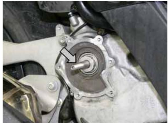
Place the calibrated punch (with preloading position).
