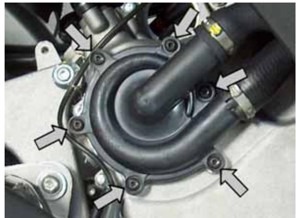
Using a 8 mm wrench, unscrew the water pump fan.
