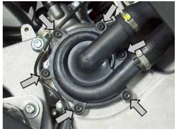
Use a 8-mm screwdriver to unscrew the water pump rotor.
