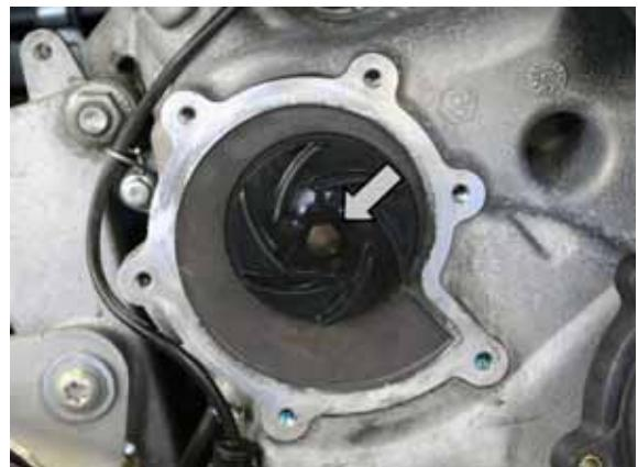
Mount the pump cover, using a new gasket, which has been greased with Vaseline.
